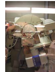
Rigaku X-ray Diffractometer for crystalline phase measurements
